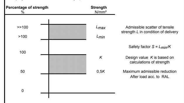
**4.** The tensile strength is tested according to 3.2.5. Results must meet the requirements of the "Material's Data Sheet".
